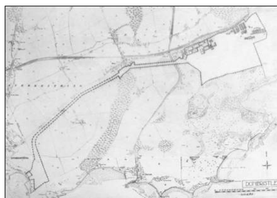
Fig. 10. Donibristle air station, Fife. The landing ground, with the technical buildings and accommodation, to the NE, was linked to the seaplane landing pier, at the SW, by a dedicated railway, on which the seaplanes were transported. (TNA AIR 452/15/312/26 vol 5)
