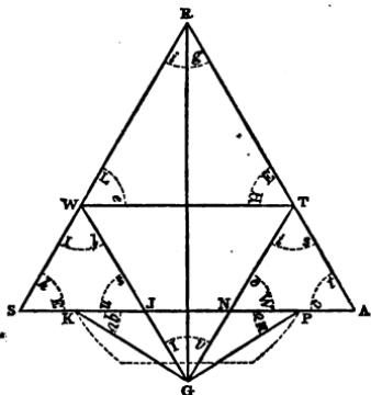
Draw the line SA any given length, which divide into five equal parts, K,J,N,P,A.
