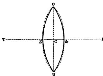
Draw O U the length of hull, which bisect at C with the line Z & produced on both sides. With  $\frac{1}{3}$ th the length of hull in your compasses, place one foot in U and the other in I, and describe the arch U O ; and, with the same distance in your compasses, place one foot in O and the other in T, and describe the arch O U, which will form the deck, Z & being the breadth of beam.
