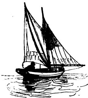
In a short rippling sea, this boat could not be stayed, although every power she possessed without oars was tried. When the helm was put down, the jib-sheet was eased off and the main-sheet hauled in, the jib-sheet was boomed out, and, when she took stern way, the helm was immediately shifted. All would not do ; she lost her way before bringing the wind right ahead, the water ceased to act upon the helm—the sea knocked off her bow, and back again she went.
